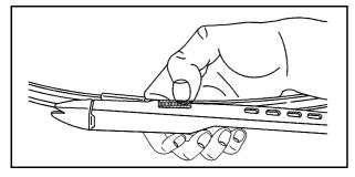
2. Squeeze the grooved areas on each side of the blade, and turn the blade assembly away from the arm connector.
